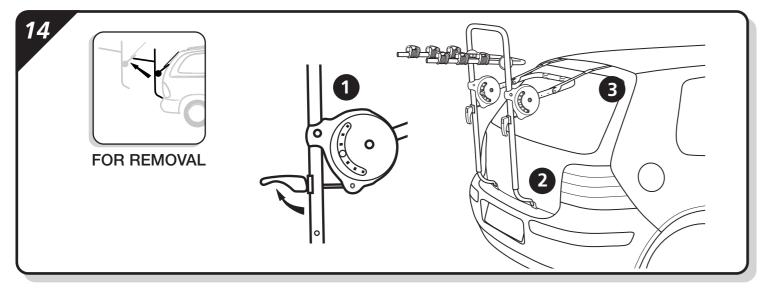
When removing the carrier from your vehicle (1) release both carrier clamping levers. (2) Unhook the feet from the bottom of the tailgate. (3) Unhook the metal clamp straps from the top edge of the tailgate.
